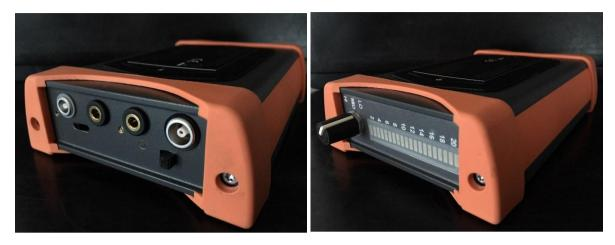
The receiver is housed in a robust Aluminum profile case that is protected by a shock absorber. The front side provides the controls and the display. The rear side provides further controls as well as all connectors.
